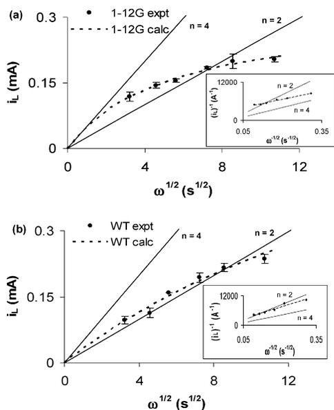
**Figure 4.** Levich plots for (a) 1-12G and (b) WT. The individual points, solid lines, and broken lines represent the experimental data, theoretical lines, and lines derived from the fit of the experimental data, respectively. The insets are the corresponding Koutecky–Levich plots, from which  $n$  and  $k_{\text{obs}}$  were derived. The  $\text{O}_2$  concentration used to generate the lines,  $2.9 \times 10^{-7} \text{ mol/cm}^3$ , is that of air-saturated buffer at  $20^\circ\text{C}$ .
